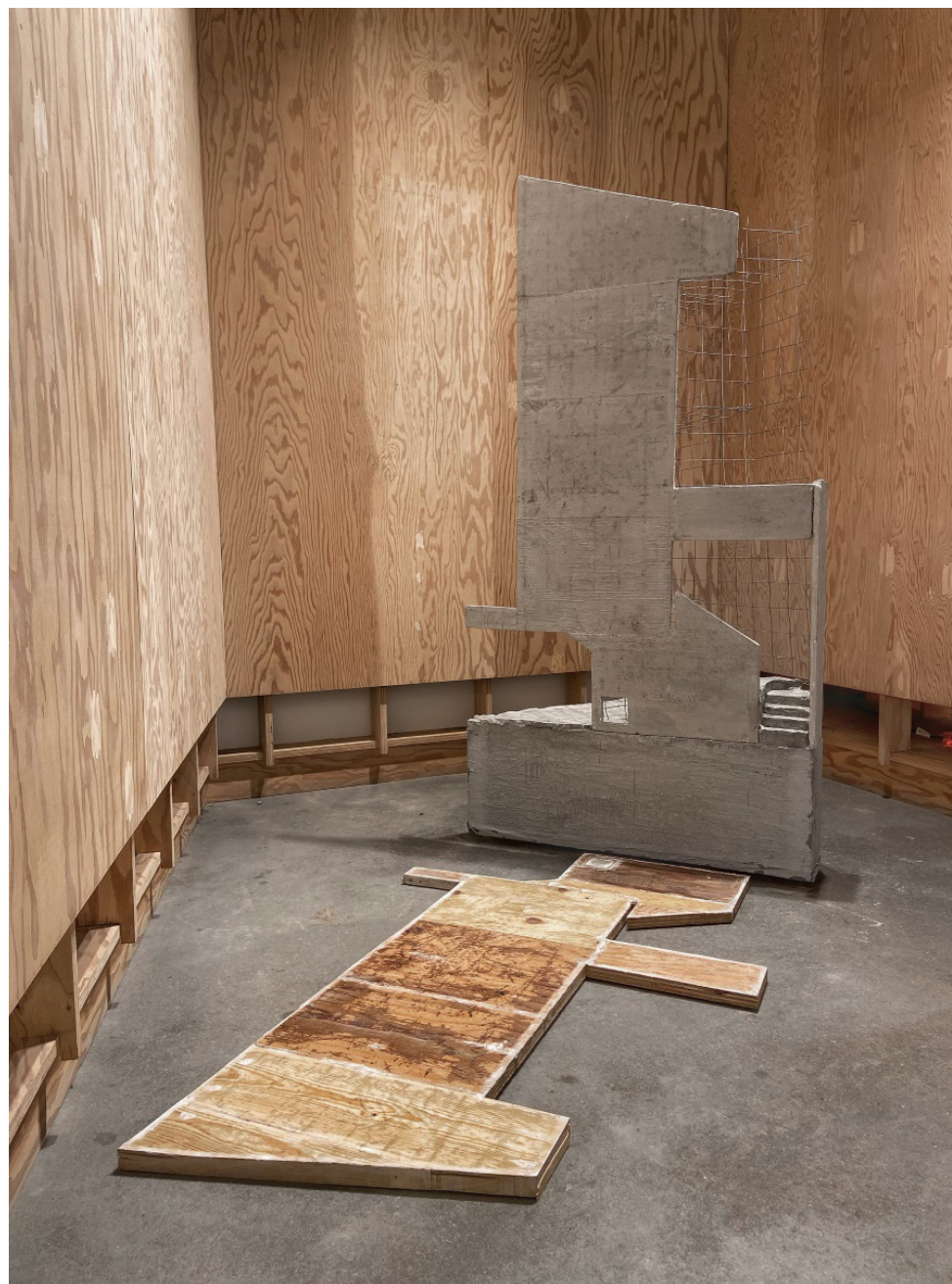
1:10 Model. Concrete, Steel Mesh, Plywood. Displayed with the plywood formwork.
