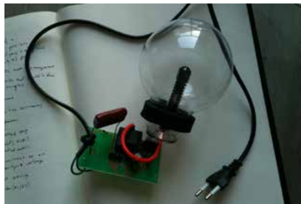
Figure 4.7: Plasma ball components (image by author, 2015)
