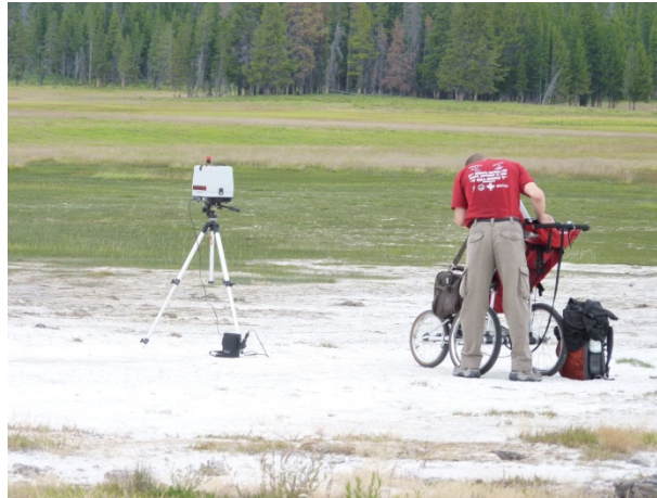
Grand Prismatic Springs (courtesy of N. Parenteau). Columnar Basalts along the roadside at Yellowstone. Bottom: Photo of Steve Ruff using a field-based version of the Miniature Thermal Emission Spectrometre (Mini-TES) at Yellowstone collecting spectra of the silica deposits (Photo: N. Parenteau).
