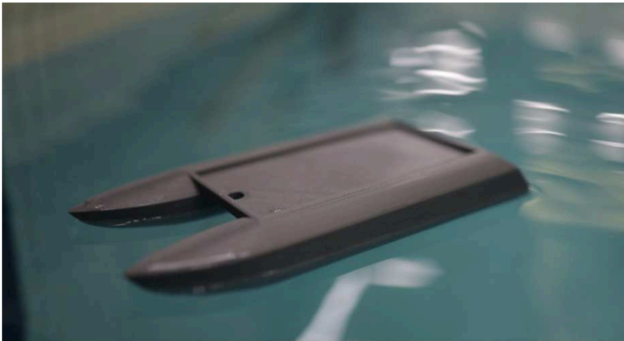
Figure F: A photo of a scaled-down mockup of the 3D printed hull in the team's pool. Note the relatively high position of the SEA LION in the water—while not explicitly weighed down like the final design will be, the PLA infill is high to simulate added mass and provide proof of concept for adequate buoyancy.
